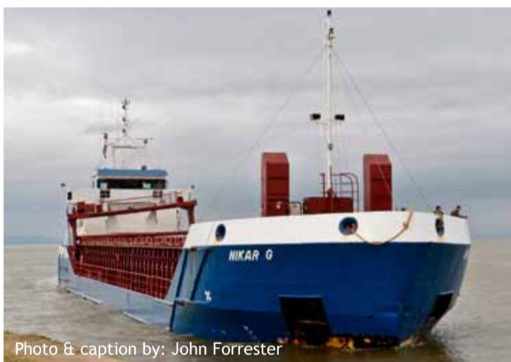
Photo & caption by: John Forrester NIKAR G arrived on 17th February after suffering storm damage in the English Channel en route from Riga, Latvia. The dislodged hold gantry crane can be clearly seen. There was also damage to telecommunication equipment.
